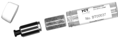
Figure 16-1: STM Sample Holder Container. (from left to right) Screw cap, Sample holder, Silica container, Sample Holder Container.
