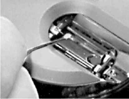
Figure 16-2: Cleaning the sample holder guide spheres
