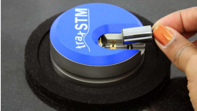
Figure 3-6: Placing the Sample Holder in the scan head
